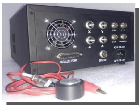
Nuline VECTRA CNC controller box is a bridge between CNC software and CNC machine. Vectra CNC is equipped with 3 Linear axis (X,Y and Z). Controller has the dedicated emergency stop push switch and supports safety limit switch by sensing the signals from limit switches from all the 3 axis. The controller comes with RPM knob to maintain the speed of spindle for different applications.
