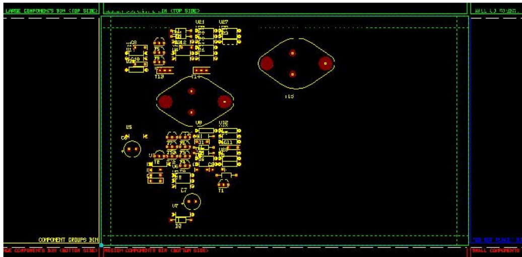
Figure: Auto Placement of the Components
