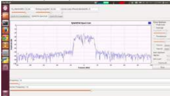
QAM 256 Rec eived Signal Spec tral Display at 1GHz
