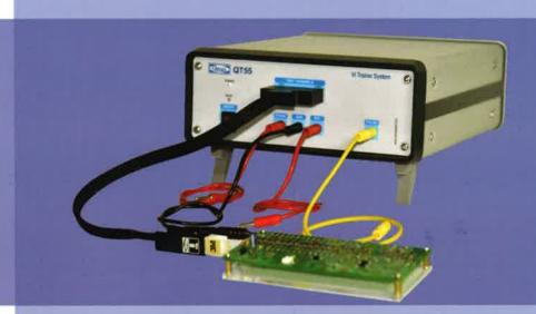
To educate the students on the basic principles of testing discrete components such as resistance, capacitance, inductance, diodes, transistors and filter circuits using voltage *vs* current (V-I) characteristics. Using this trainer basic power electronics components such as MOSFETs, diacs, triacs, SCRs and opto couplers can also be tested using trigger pulse & signature method.
