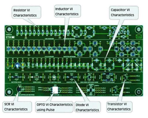
By doing these VI Characteristics experiments, one can understand the concepts of analog signature analysis and its test methods. It is also called as VI-Characteristics. By this students will come to know how to learn the characteristics of each and every passive and active components using test engineering practical trainer kit.
